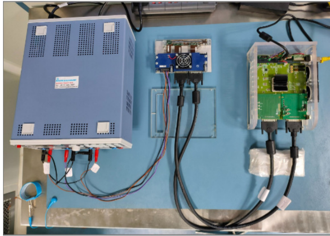
Fig 1. Phase-II Tracker module test setup in the HENPP cleanroom.
