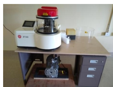
Fig. Sputter Coater System
